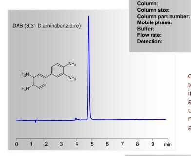
BIST<sup>™</sup> B+ 4.6 × 100 mm, 5  $\mu$ m TBP-46.100.0510 Gradient MeCN - 80-30%, 10 min H<sub>2</sub>SO<sub>4</sub> - 0.2% 1.0 mL/min UV 280 nm
